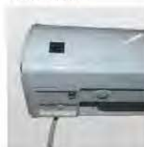
IR Sensor and Manual Override
